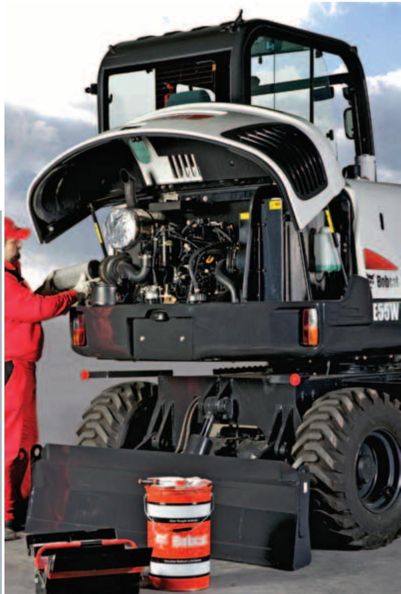
You can easily reach routine maintenance service points, including filters and air bleeding system, thanks to the large tail gate and the transversely mounted engine.
